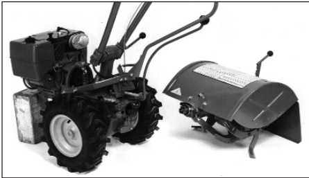
Figure 4-21: PTO Power Unit and tine attachment.
